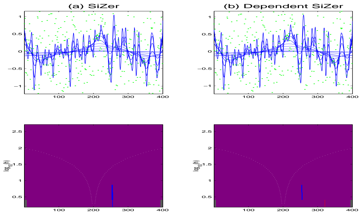
Figure 5: (a) Original SiZer of simulated independent errors. Almost all pixels are purple in the lower panel, which is consistent with the given model. (b) Dependent SiZer of simulated independent errors. It shows that dependent SiZer gives the same result as that of conventional SiZer when the errors are white noise.
