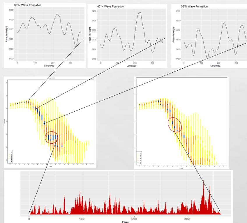
Figure 1. Workflow for Sequential Filtration. Individual waveforms are analyzed to form seahorse plot summaries, which form a time series of relative evidence for a wavenumber-5 formation
